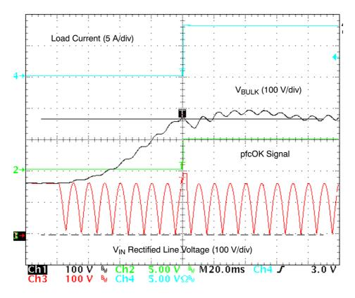
Figure 8. Startup Phase at 120 Vrms and  $I_{OUT}$  = 8 A
