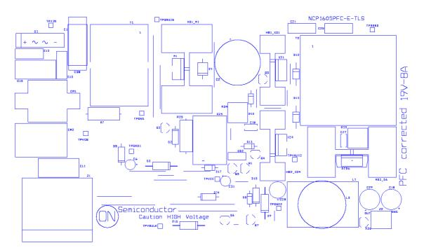
Figure 4. PCB Layout - Silkscreen Top
