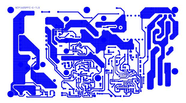
Figure 6. PCB Layout - Bottom Layer
