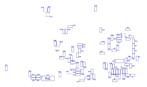
Figure 5. PCB Layout - Silkscreen Bottom
