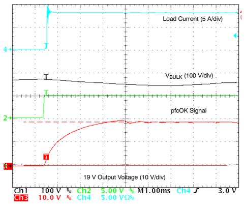
Figure 10. Startup Phase at 120 Vrms
