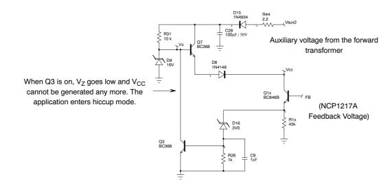
Figure 13. Circuit for Overload Protection
